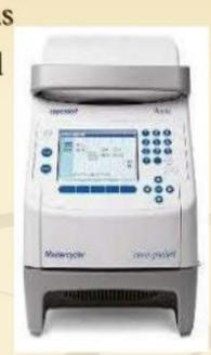
Use arrow keys to select the program you want to run. Press "ENTER". The program will ask you what kind of tube you're using and the reaction volume; select the tube with the "SELECT" button, enter the volume on the number keypad; hit "ENTER". -- While the program is running, you can use the "OPTION" key to check how much longer you have to wait.
