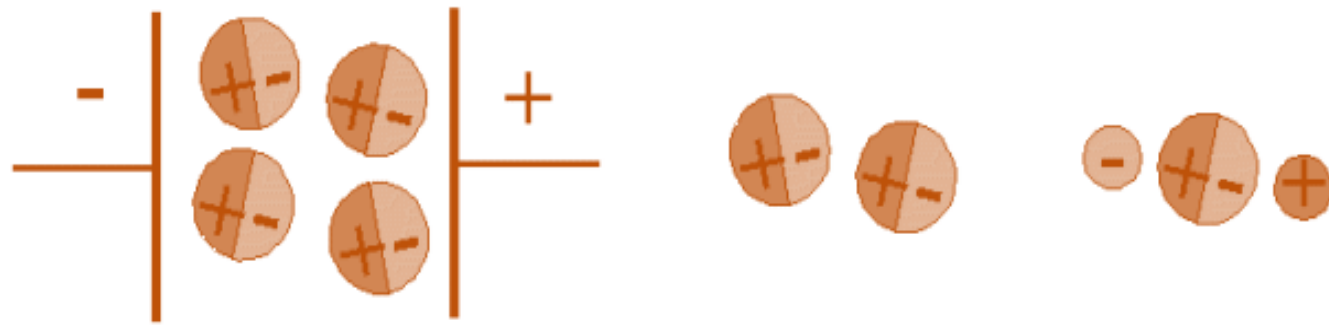
Figure 2: Polar molecules align themselves in an electric field (left), with respect to one another (middle), and with respect to ions (right)
