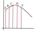
The area under the first parabola ABC =  $(y_0 + 4y_1 + y_2) \times dx/3$ The area under the first parabola CDE =  $(y_2 + 4y_3 + y_4) \times dx/3$
