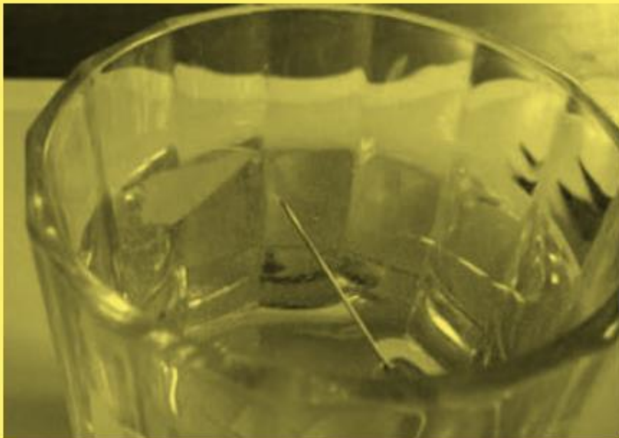
FIGu r e 1.4 An iron needle floats on the surface of water ( only if carefully placed; otherwise, it should sink due to gravity forces ).
