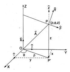
In cylindrical polar coordinates the coordinates of a point P is represented by  $(\rho, \phi, z)$ . The position vector of P is given by
